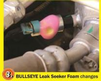
precisely locates the leak site area
